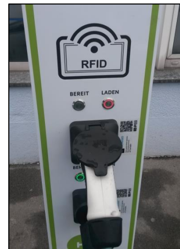
Figure 3: Charging station with RFID field (Source: im-plan-tat)
